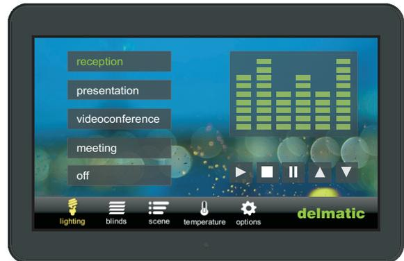
The **touchpanel** is fully software configurable and can include custom graphics and logos, multiple function sub-menus as well as configuration options and user preferences.
